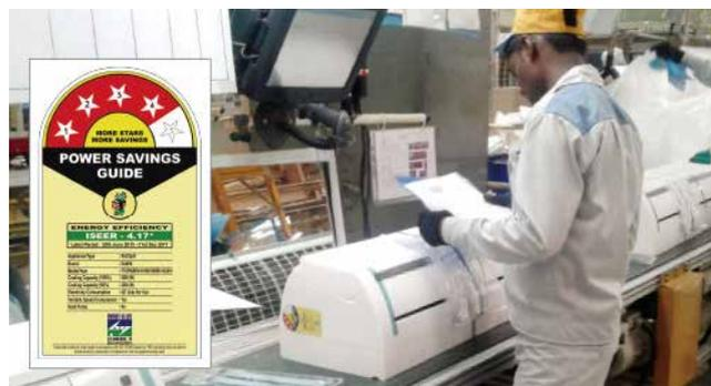
Air conditioner affixed with new energy label based on index for proper evaluation of inverters
